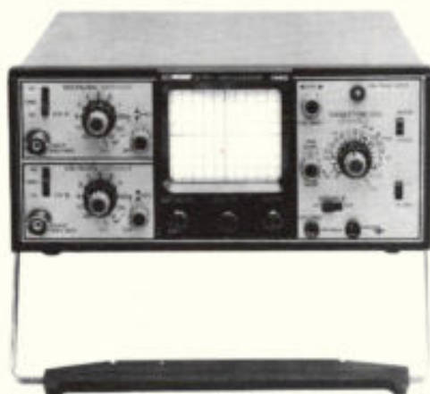
Model 3020 Sweep/Funktie generator (0,02 Hz - 2 MHz).
